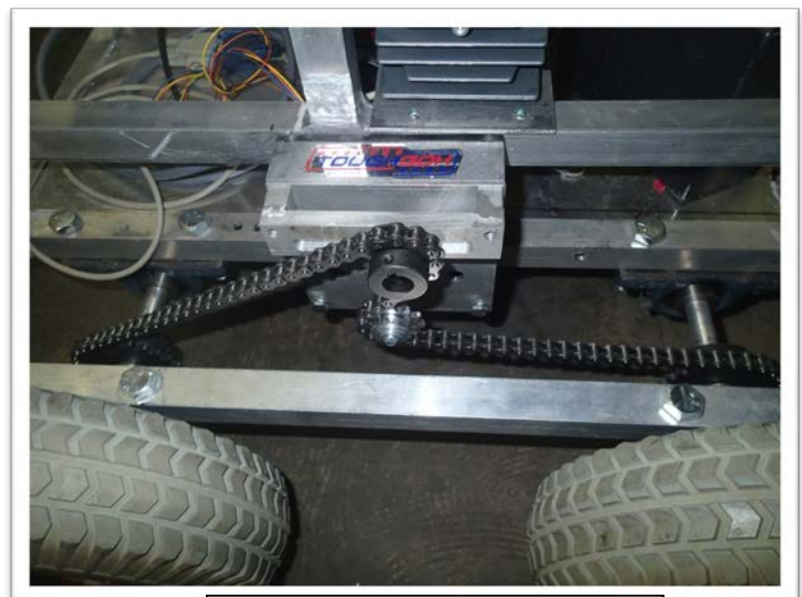
Custom chain tensioning system
